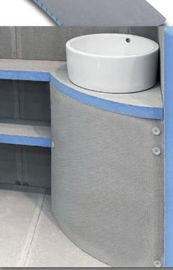
You can also bend the curved Multiboard with the slits on the outside. If this is done then a flexible cement based tile adhesive needs to be used to fill out all of the slits on the surface and a sheet of Marmox fibreglass mesh needs to be layed over.
